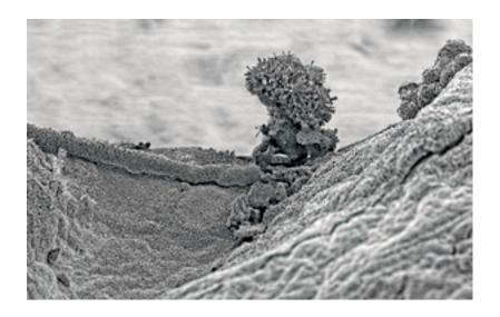
NANOSCAPES: Zinc Oxide Glen Inside a tube furnace at 500–600 °C, shrub-like forms take shape on a grass of zinc oxide that has grown atop a zinc foil. (C&EN Vol. 86, No. 47, November 4, 2008)
