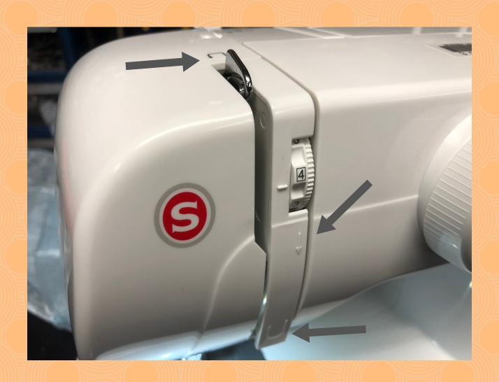
Use the arrow guides on the machine to thread the string until you're ready to insert it through the needle
