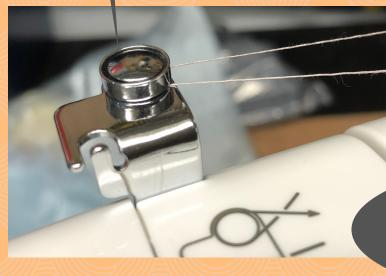
Wrap the thread around the new bobbin and place it onto this nob snuggly
