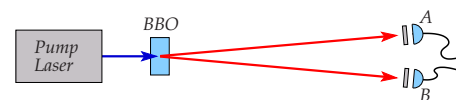
Fig. 2. A pump laser undergoes spontaneous parametric down conversion in a \beta -barium borate (BBO) crystal. The down-converted light is filtered before hitting the couplers. Although most of the pump laser passes unaffected through the crystal, we omit this beam from the diagram for clarity.
