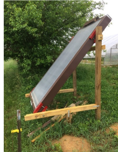
Figure 3. Solar panel used to heat the digester
