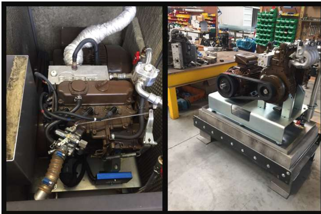
Kubota CHP belt drive system, either 11 or 22kW. Photos by Martin Energy Group
