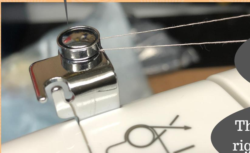
Wrap the thread around the new bobbin and place it onto this nob snugly
