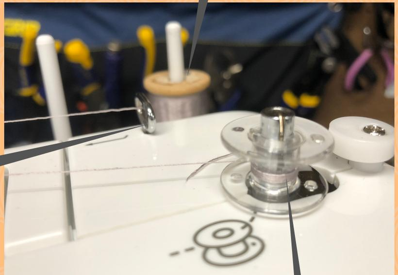
Use the metal pieces to thread the string and wrap it around the screw
