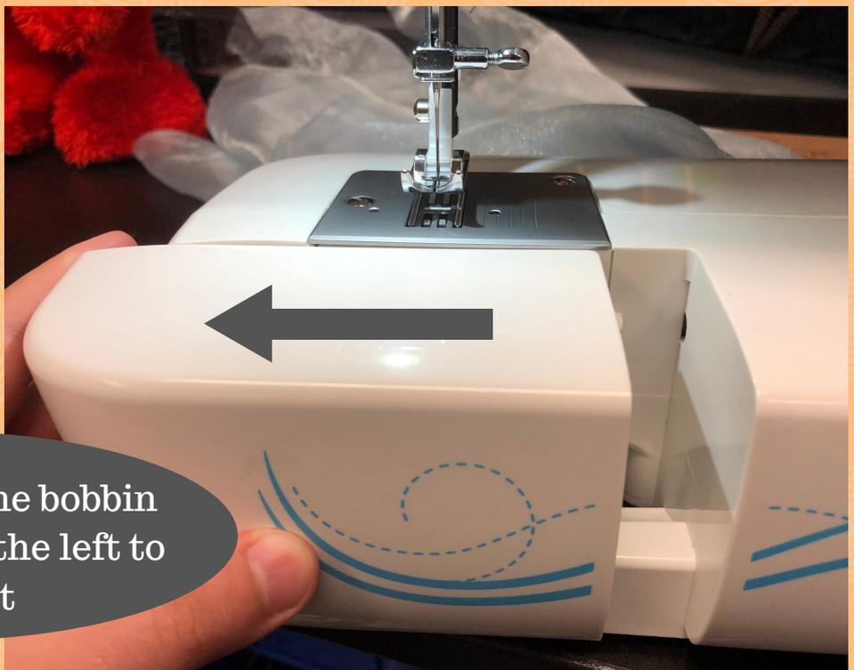
Carefully slide the bobbin compartment to the left to remove it
