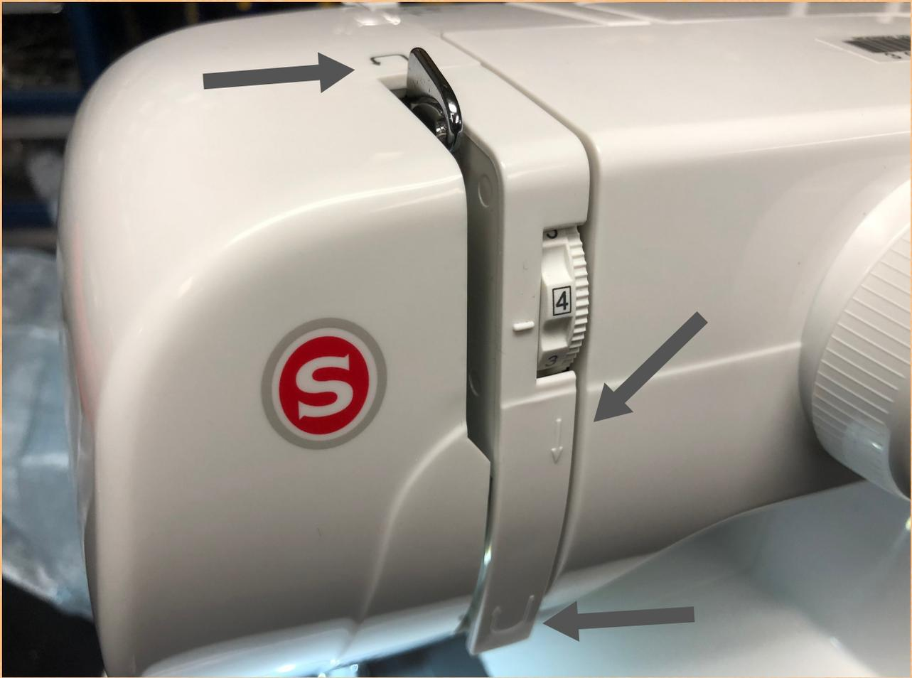
Use the arrow guides on the machine to thread the string until you're ready to insert it through the needle
