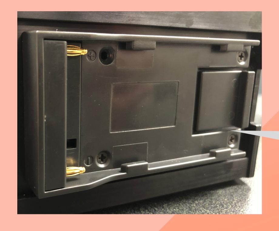
Batteries are installed on the rear of the device
