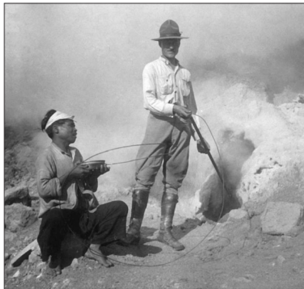
Measuring the temperature of the fumaroles at the Papandayan volcano. 1924.
